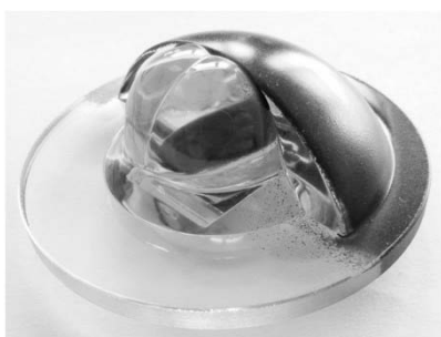
FIGURE 6. Photograph of real SOE with metalized cavity. Paint applied on the cavity surface to protect Ag metallization.
