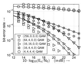
Figure 5: BER with PA (dotted line) and without PA (solid line) when using the transmission modes introduced in Tab. 1 and transmitting 8 bit/s/Hz over correlated frequency non-selective channels.
