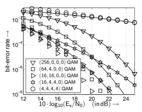
Figure 2: BER with PA (dotted line) and without PA (solid line) when using the transmission modes introduced in Tab. 1 and transmitting 8 bit/s/Hz over uncorrelated frequency non-selective channels.
