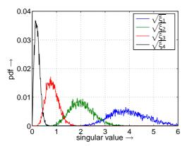
Figure 4: PDF (probability density function) of the layer-specific amplitudes  $\sqrt{\xi_\ell}$  for correlated frequency non-selective MIMO channels.
