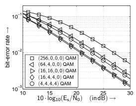
Figure 6: SVD-based user-specific BERs without PA when using the transmission modes introduced in Table 1 and transmitting 8 bit/s/Hz over uncorrelated frequency non-selective channels.
