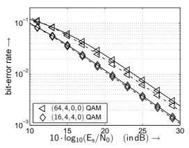
Figure 7: User-specific BERs with PA (dashed line) and without PA (solid line) when using the transmission modes introduced in Table 1 and transmitting 8 bit/s/Hz over uncorrelated frequency non-selective channels.
