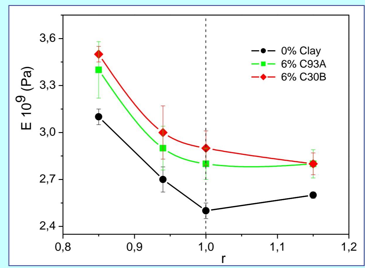
Glassy state: the highest modulus is observed in epoxy-rich compositions ( $r < 1$ ).
