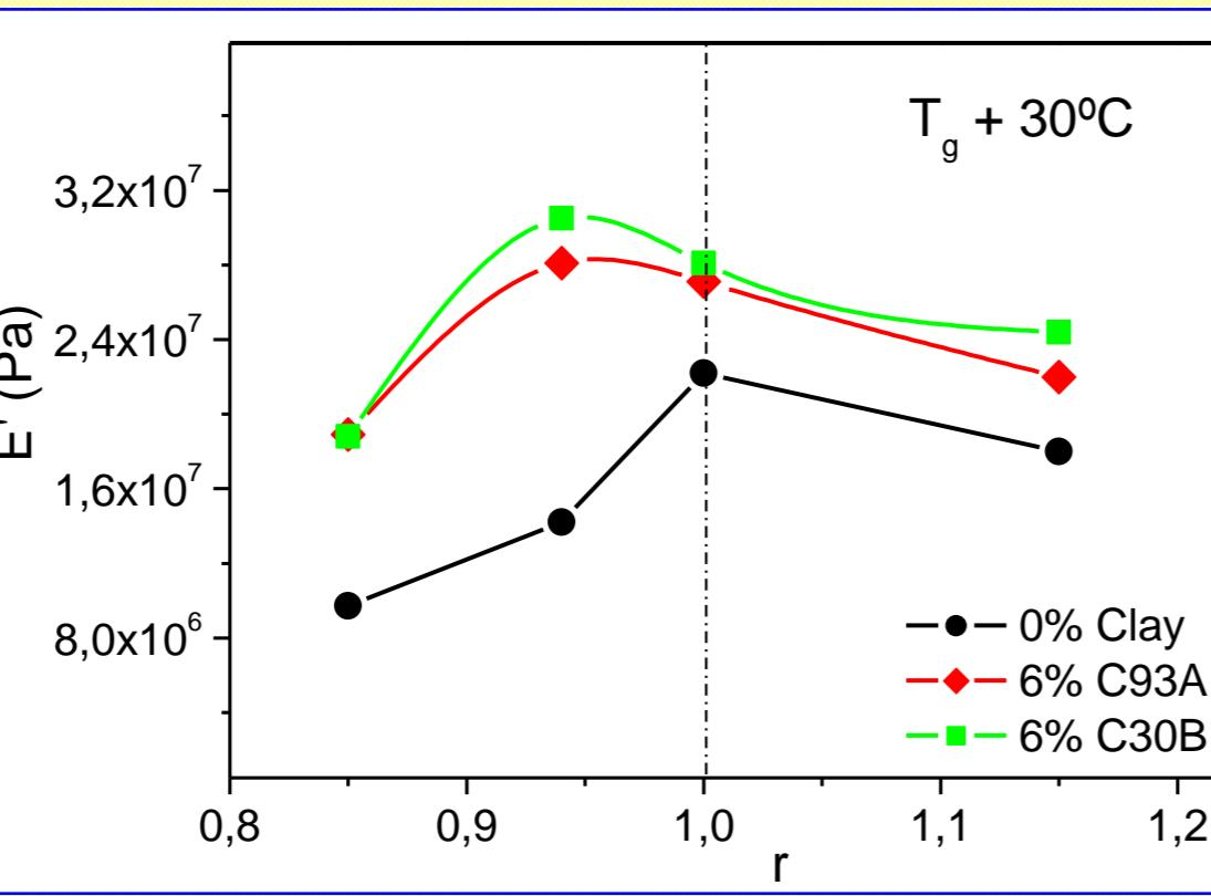
Rubber state: clay-epoxy nanocomposites have higher  $E'$  rubber than neat epoxy thermosets for  $r \leq 0.94$ , but lower for  $r > 1$ .
