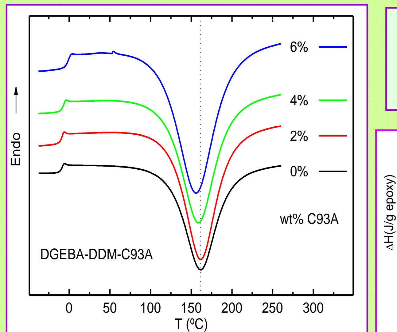
C93A-DGEBA-DDM and C30B-DGEBA-DDM the exothermal peak temperature shifts to lower values → the clays accelerate the curing reaction
