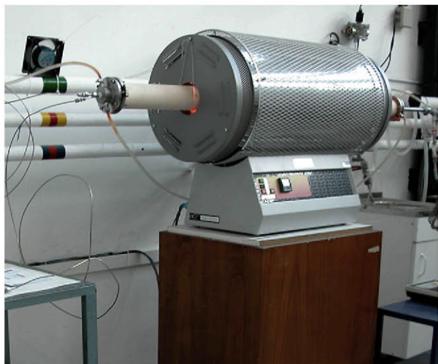
Fig. 5 – Horizontal furnace for SiC experiments.
