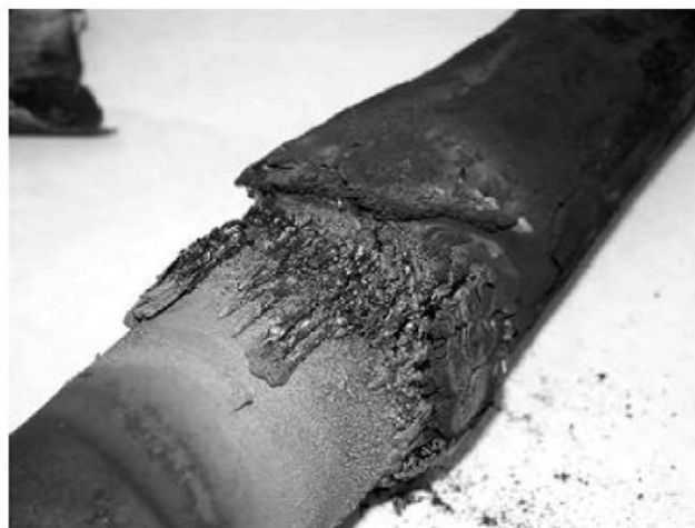
Fig. 4 – Carbon depositions on the external surface of the graphite tube.
