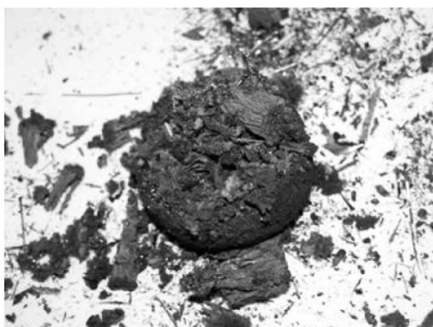
Fig. 3 – Carbon plug specimen obtained at Gr-4 experiment.
