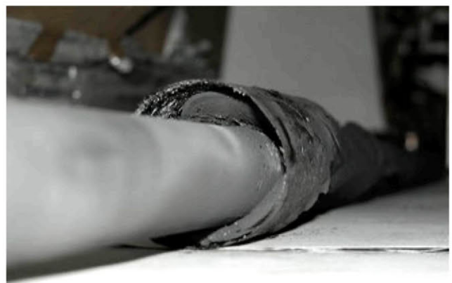
Fig. 12 – Graphite tube after 3 h tests for the experiment Gr-15, with a non-porous tube.
