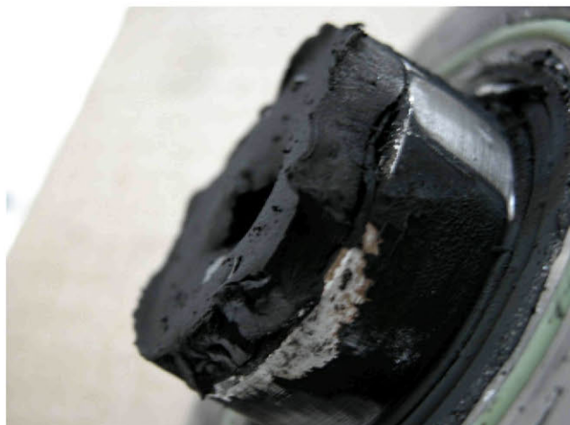
Fig. 6 – Soft carbon plug at 1200 °C.
