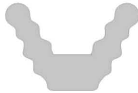
Figure 10. Cross section of rubber ring in the resilient wheel with V-ring.
