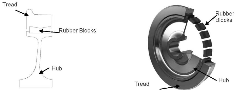
Figure 5. Cross section and 3D view of the resilient wheel with rubber blocks
