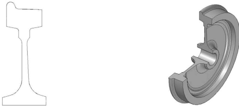
Figure 3. Cross section and 3D view of the monobloc wheel
