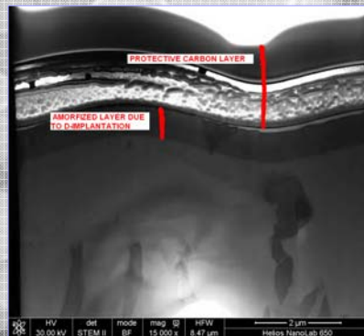
Cross sectional SEM image of an as-implanted Li_2TiO_3 lamella prepared by FIB.
