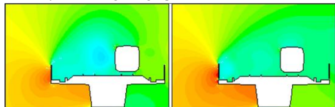
Figure 5: The barrier of the left side is simple of 1.75m. The barrier of the right is 2m and has a small gap. This one, reduces considerably the depression between the barrier and the train (blue areas).
