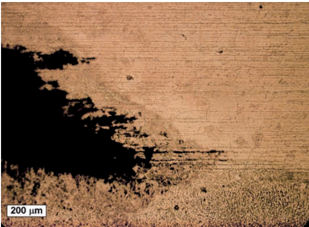
Figure 5. Pitting corrosion on the base-metal side. The corrosion has progressed along the lamination bands of the base metal.
