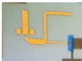
Fig. 6.23: Detail of one output port with ground patches for probe positioning.
