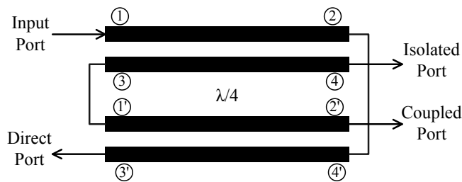
Fig. 3.3: Schematic of a tandem coupler.
