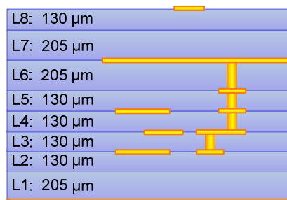
Fig. 6.1: LTCC layer structure using DuPont-951 substrate.
