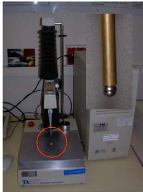
Figure 2. Texture Analyser TX2 machine and detail of the compression tool used for maize particles
