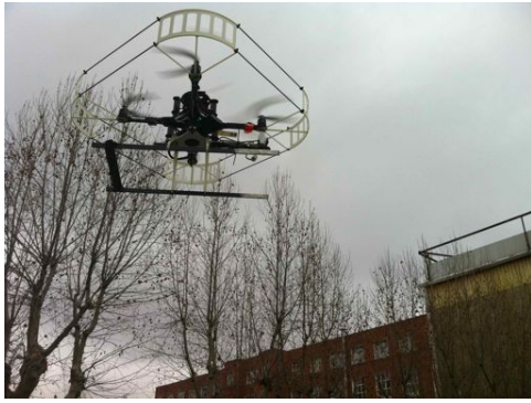
Fig. 3. CVG-UPM [17] Pelican QuadCopter testbed used for sense and avoid experiments
