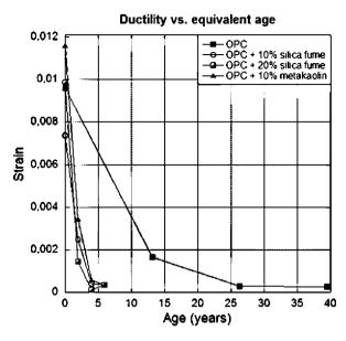
Fig. 8. Ductility vs. equivalent age.
