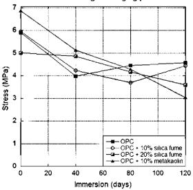
Fig. 2. Tensile strength vs. aging period.
