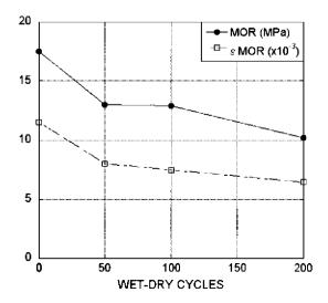
Fig. 11. Effect of wet-dry cycles in OPC GRC.
