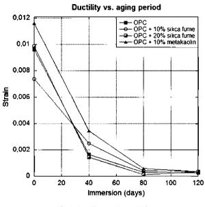
Fig. 3. Ductility vs. aging period.
