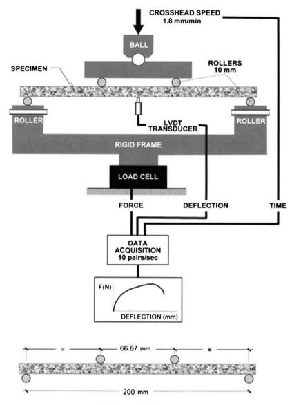
Fig. 4. Four point bending test sketch.
