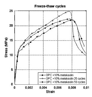
Fig. 6. OPC GRC with 10% metakaolin four point bending test stress-strain curve.
