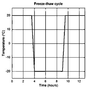
Fig. 1. Freeze-thaw cycle.
