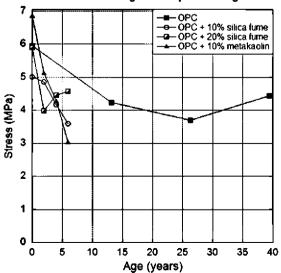
Fig. 7. Tensile Strength vs. equivalent age.
