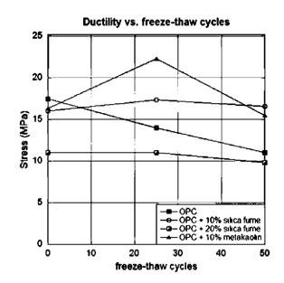
Fig. 9. Bending vs. freeze-thaw period.
