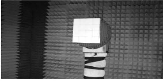
Fig 8. Measurement of an X-Band array antenna in spherical near-field.
