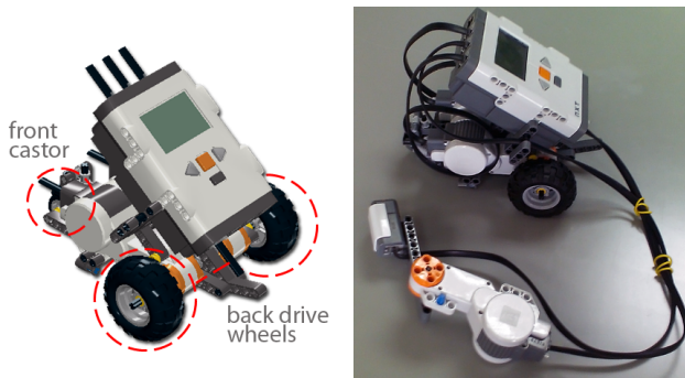
Figure 6: Vehicle prototype fully assembled.
