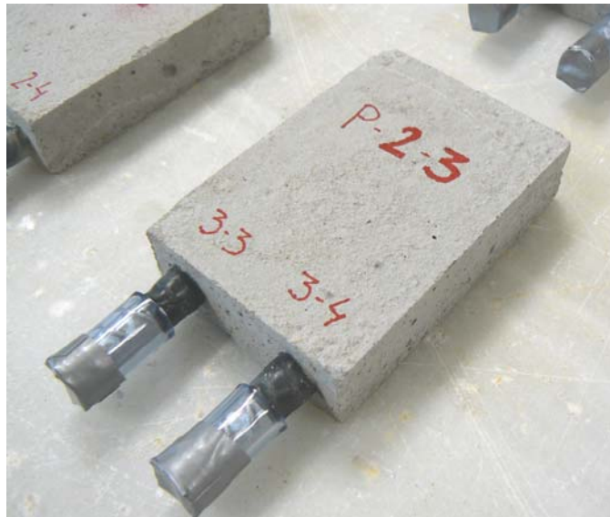
Figure 1: Reinforced concrete specimen embedding two stainless steel reinforcements Ø8 mm wide.
