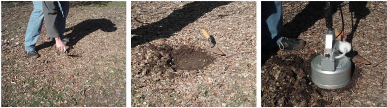
Fig. 2. The CO 2 diffuse flux clearance and measurement process.
