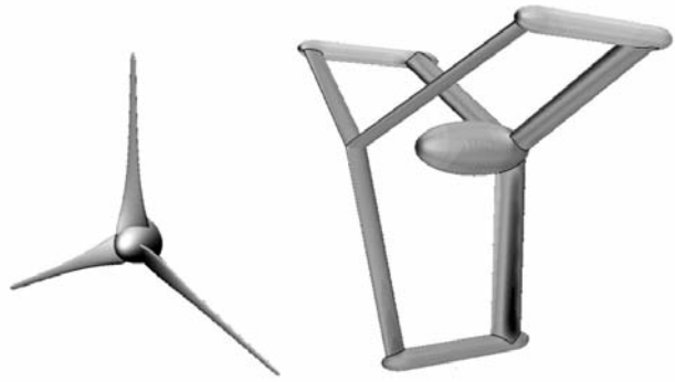
Figure 6. Preliminary physical and CFD models of the GESMEY rotor and structure.
