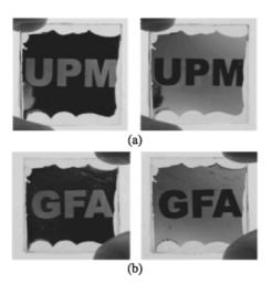
Fig. 3. Pictures of a device when a polarizer is placed in front of the LC cell (a) and when a polarizer is placed behind LC cell (b). Complementary images are obtained when a polarizer is ro-tated 90°.
