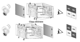
Fig. 2. Schematics of security device operating principle. Dichroic dye absorbs the light depending on orientation of LC molecules and polarization of light. Situation of polarizer determines which of two latent images is visible. Only an image generated on a substrate closest to a polarizer is seen.
