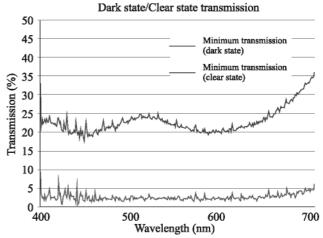
Fig. 7. Transmission obtained for one standard manufactured device in the case of dark state and clear state.
