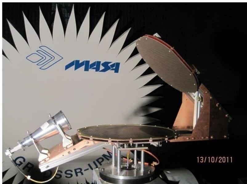
Fig. 4-58. Installation of the breadboard in the compact range anechoic chamber
