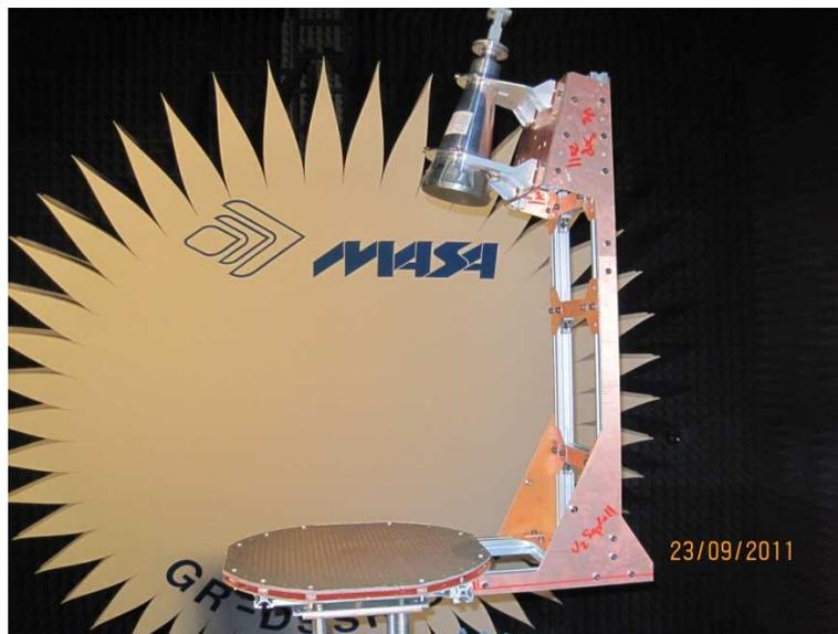
Fig. 4-55. Sub reflectarray breadboard in the compact range anechoic chamber
