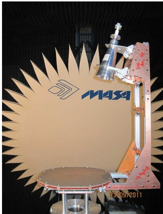
Fig. 4-54. Sub reflectarray breadboard
