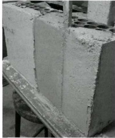
Figura 2 Two layers of 10 mm each applied on brick base
