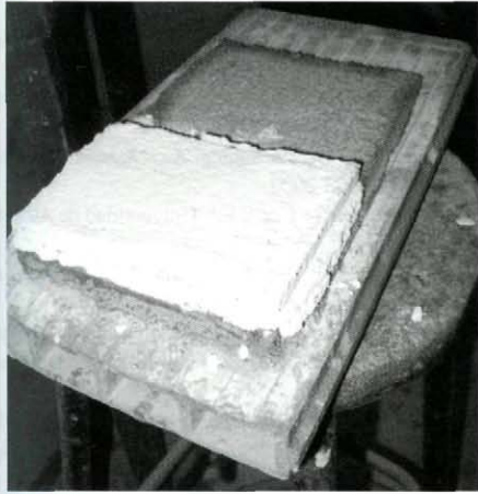
Figura 1 Mortars applied on the brick wall constructed for it
