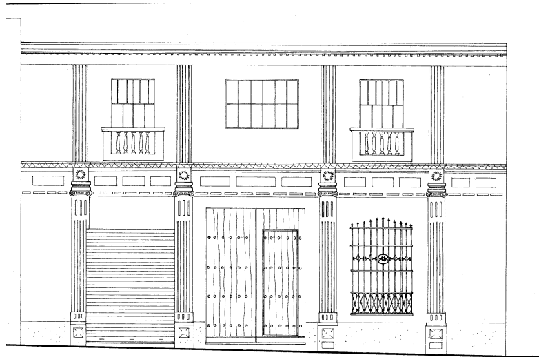
Fig. 3. Façade with two different age floors and left window converted into door.
