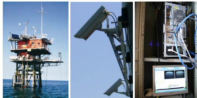
FIGURE 1. Left: off-shore platform “Acqua Alta” in the Northern Adriatic Sea, near Venice. Center: pair of synchronized cameras for monitoring the ocean climate from the platform. Right: WASS hardware installed at the platform for recording stereo videos of ocean waves.
