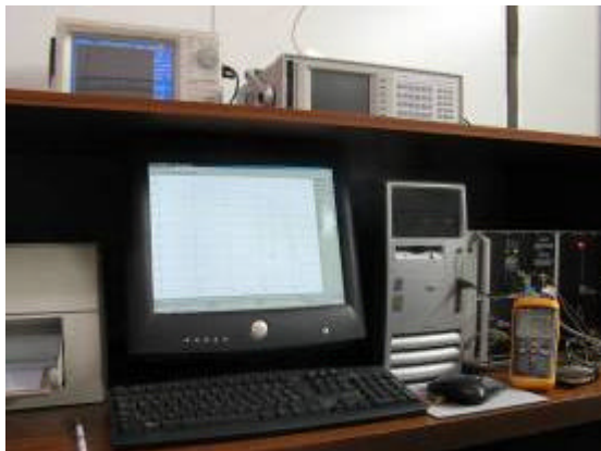
Figure 3: some of the external elements of the solar simulator: computer, electronic load and temperature indicators.
