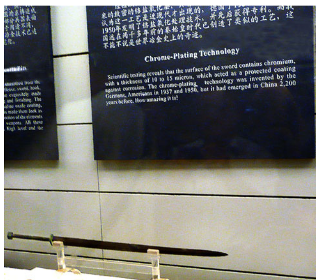
Fig. 1 2200-year-old sword coated with 10-15 \mu\text{m} of Cr found in Emperor Qin Xi Huang's mausoleum in Xi'an, China
