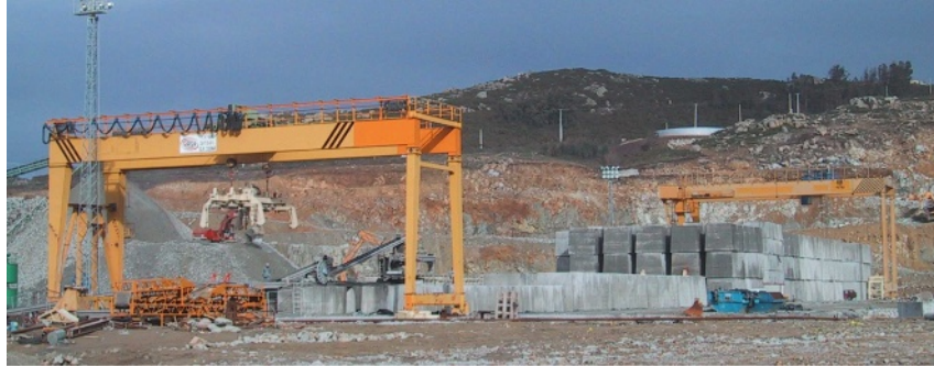
Figure 13. Close-up of the gantries used to move the blocks in the yard
