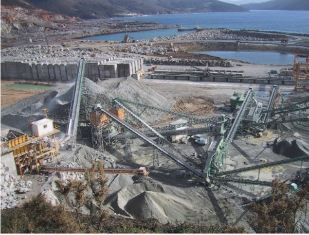
Figure 8. Aggregate manufacturing plant: at the end of the block yard and the auxiliary quay
