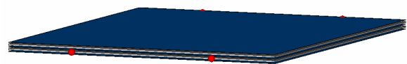
Figure 18. SEA model of the ARA-MK3 solar array in stowed configuration considering the three wings, the two air layers and only connection between contiguous wings through hinges on the lateral side of the wings
