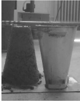
Fig. 4. Photographs of the Abrams Cone and compressive testing machine (EN 12350-1/2/3:2006; EN 12390-1/2/3:2001).
