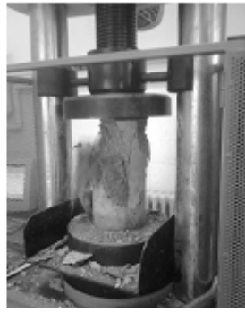
Fig. 4. Photographs of the Abrams Cone and compressive testing machine (EN 12350-1/2/3:2006; EN 12390-1/2/3:2001).
