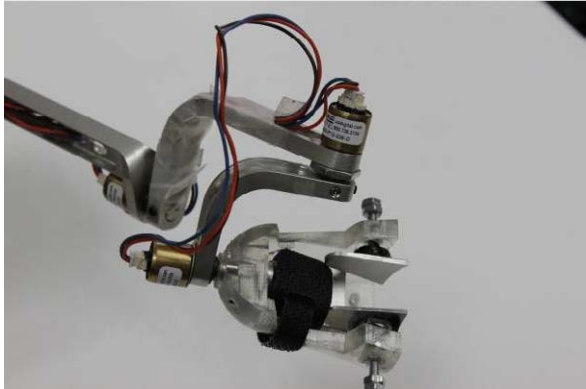
Fig. 2. Thimble attached to the gimble placed at the end of the parallel-series structure. The thimble is attached to the finger by using the screws to press the metal sheets.
