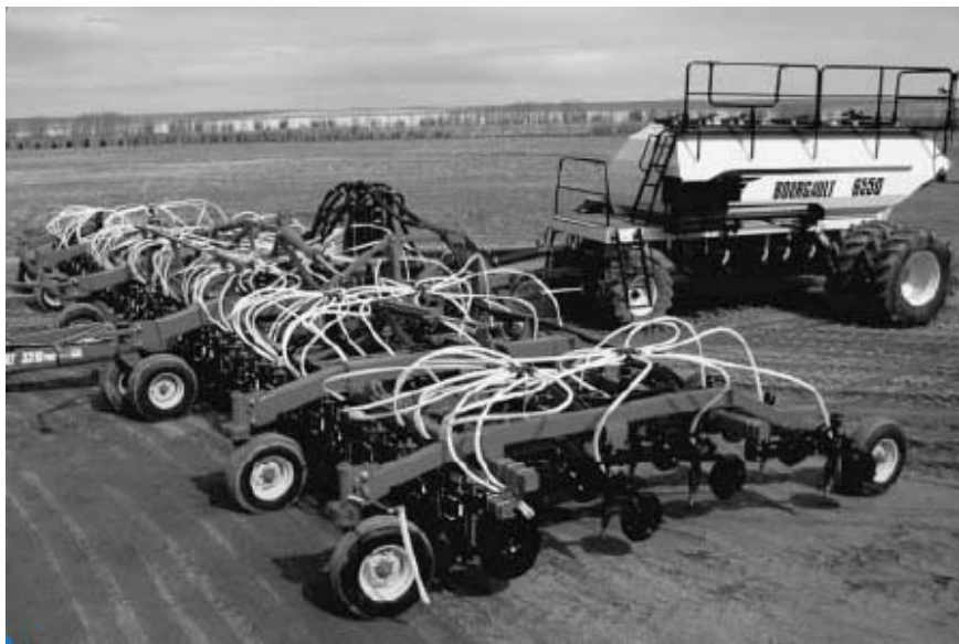
Figure 1. 3310 Paralink Hoe Drill. AE50 outstanding innovation in 2007. http://www.asabe.org/resource/ae5011entry.html
