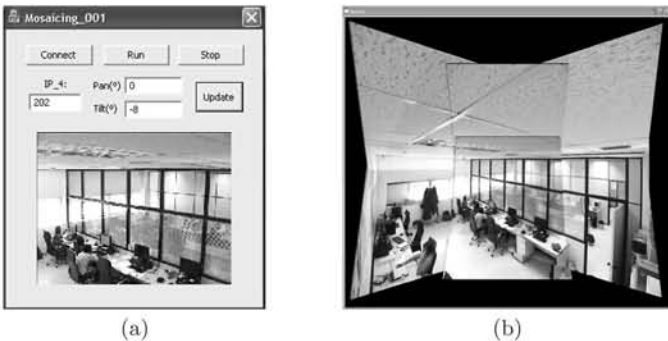
Figure 3. Indoor example. The current view (a) is pasted into the mosaic (b) according to its estimated rotation and camera calibration.
