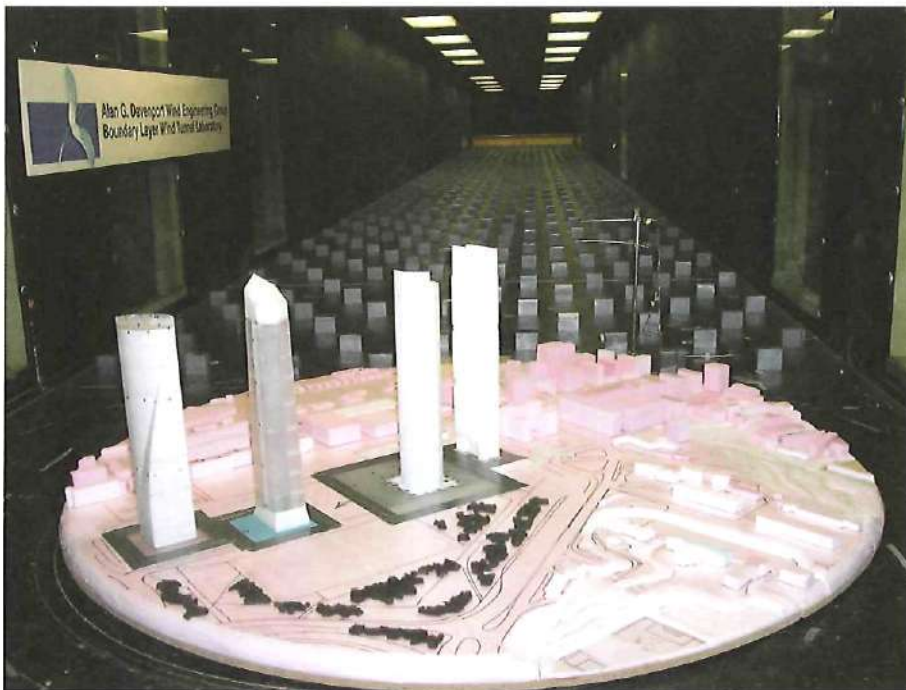
△ Figure 12 Boundary layer wind tunnel tests of the four towers at the University of Western Ontario, Canada
