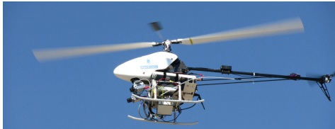
Fig. 6. COLIBRI III Electric helicopter UAV used for pose estimation tests.
