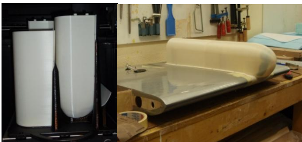
Fig. 16. Prototype IV manufacturing process. Fairing, placed and fixed onto wing
