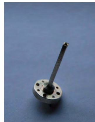
Fig. 6 WR-10 waveguide as a measuring probe.
