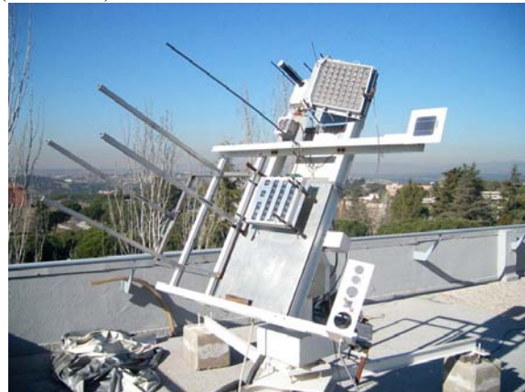
FIGURE 2: Two-axis sun tracker installed on the flat roof of the Instituto de Energía Solar – Universidad Politécnica de Madrid (IES-UPM).
