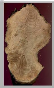
At least one section was obtained from each specimen. In each sample a minimum of two or three radios were measured and crossdated (with the equipment and application LINTAB Win and TSAP).
