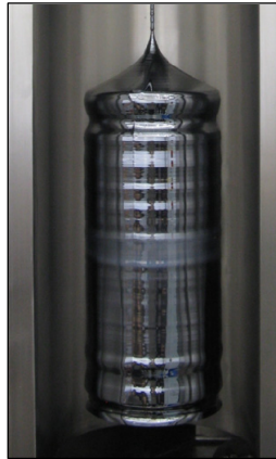
Figure 2. Silicon ingot growth through the Cz process
