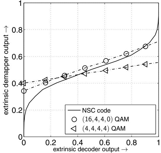
Figure 8: User-specific EXIT chart for an effective throughput of 4 bit/s/Hz when using anti-Gray mapping on all activated MIMO layers ( $10 \log_{10}(E_s/N_0) = 7$  dB) and the half-rate NSC code with the generator polynomials of (7,5) in octal notation.
