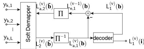
Figure 3: Iterative demodulator structure.
