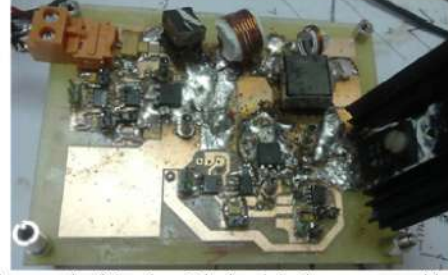
Fig. 11. Photograph of the class E isolated dc-dc converter with one output
