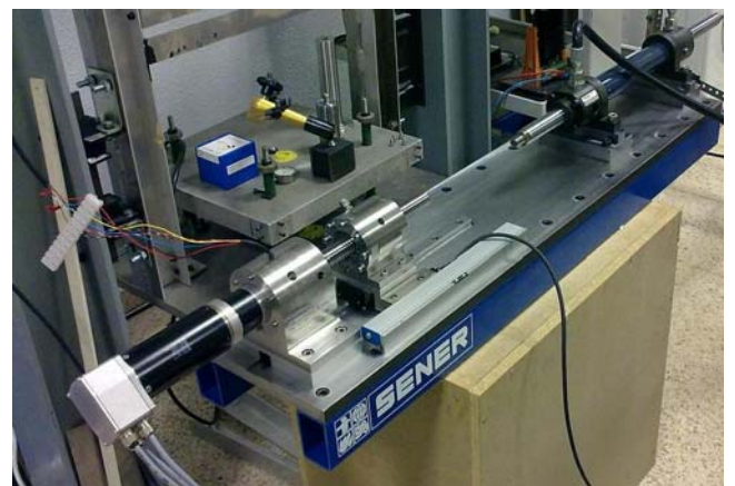
Figure 9. Screw/ Nut assembly test rig (set up)
