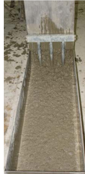
Fig. 2 Concrete in L box after testing.
