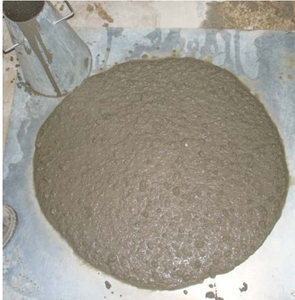
Fig. 1 “Slump-flow spread” after slump flow test.
