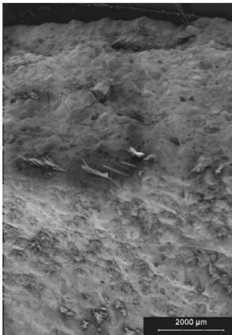
Fig. 15. GRC aged 120 days with 4% acrylic resins.
