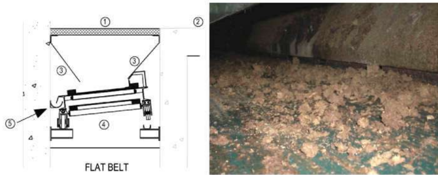
Fig. 1. Transversal section of flat belt (1, slatted floor; 2, concrete floor; 3, deflector; 4, belt; 5, gutter) and droppings clusters on the belt.
