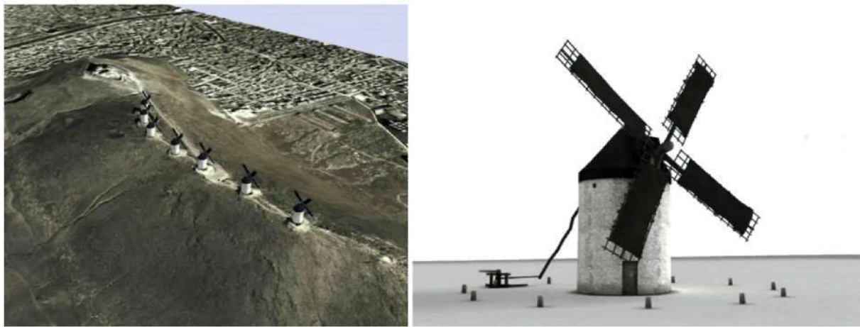
Fig. 10. DEM with superimposed digital orthophoto and windmill 3D model.
