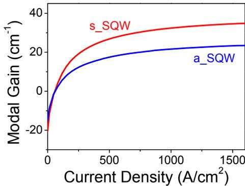
Fig. 13: Calculated modal gain vs current density characteristics for the s-SQW and a-SQW epitaxial designs.
