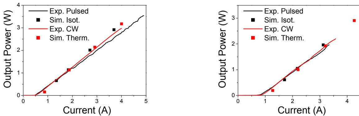
Fig. 5. Experimental and simulated power-current characteristics for 4° (left) and 6° (right) devices in pulsed and CW driving conditions.
