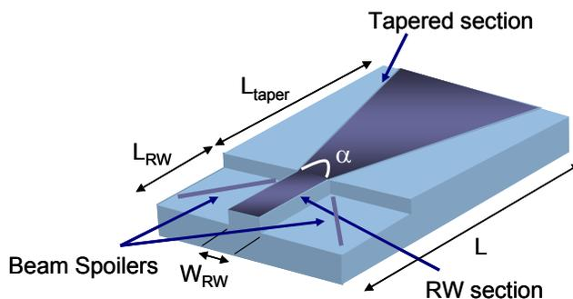
Fig. 1 Schematics of a gain guided tapered laser.
