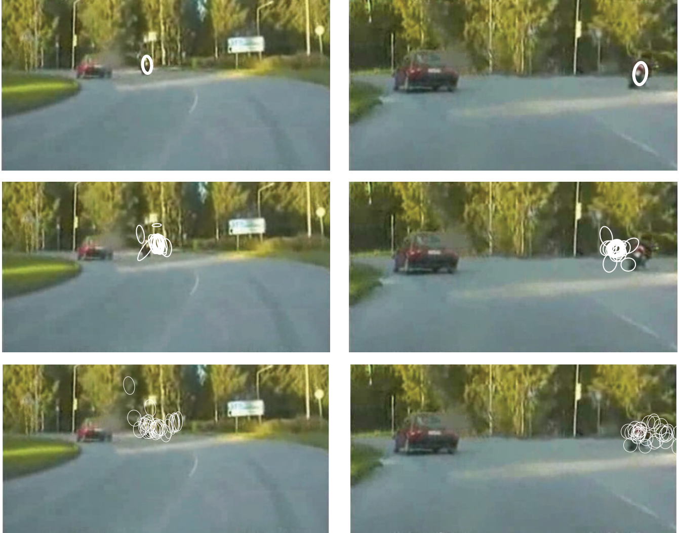
Figure 2. Tracking results in a motorbike chase from a camera mounted on a car. The first row shows the estimation of the object state represented by a white ellipse for two different frames. The second row shows candidates of the object state taking only into account the camera dynamics. The third row shows the modified candidates of the object state using also the object dynamics.
