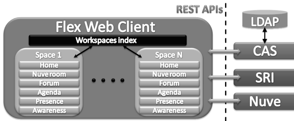
Figure 1: CollawareSoft architecture where the web client communicates with server modules through REST APIs
