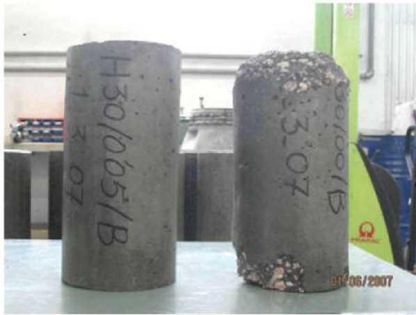
Fig. 14 Specimens C30-0.05-W and C30-00-W after 300 freeze-thaw cycles.
