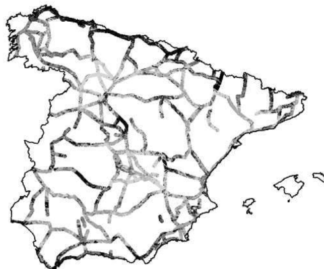
Fig. 2. Potential impact map: result of screening model for assessing the impact of PEIT infrastructures on Spanish biodiversity and environment (only 12-km-wide corridors around each of the new infrastructures in the plan are defined and mapped). Metadata: European projection standard Lambert Equal Area and Datum ETRS89. 100 m pixel-raster maps. Colour codes: compatible potential impact = light grey; moderate potential impact = grey; severe potential impact = dark grey; critical potential impact = black.
