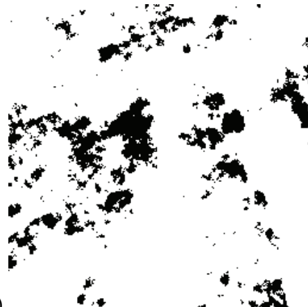
Fig. 3. The obtained results for the K-means method: (a) the image segmented with nine clusters; and (b) the binary image obtained from the segmentation process, where 0 value corresponds to the pore space class and 1 value corresponds to the soil solid class.
