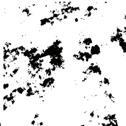
Fig. 4. The obtained results for the fuzzy C-means method: (a) the image segmented with nine clusters; and (b) the binary image obtained from the segmentation process, where 0 value corresponds to the pore space class and 1 value corresponds to the soil solid class.
